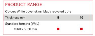
Tolerances: -0 to +5 mm on width and -0 to +10 mm on length.
